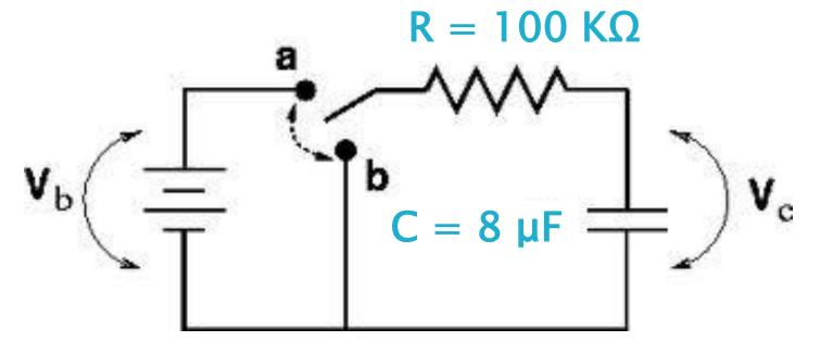
$R = 100 \text{ K}\Omega = 100 \text{ x } 10^{3} \Omega$   $C = 8 \mu\text{F} = 8 \text{ x } 10^{-6} \text{ F}$   $\tau = (100 \text{ x } 10^{3})(8 \text{ x } 10^{-6}) = 0.8 \text{ seconds}$  $\tau = 800 \text{ ms}$
