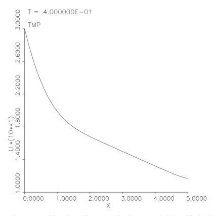
c. Repeat problem 2a with no conduction,  $\kappa=0$ . Now this is the hyperbolic transport problem of Example 8.1 (p153), and there should now be "no" boundary condition at the outlet, since it is first order in space. Note that without conduction (diffusion of heat), the discontinuity in the derivative is not smoothed out now, but simply transported forward with velocity v.
